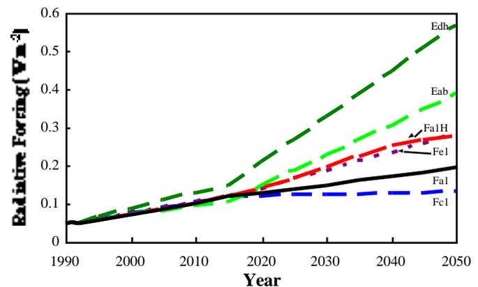
**Figure 3:** Estimates of the globally and annually averaged total radiative forcing (without cirrus clouds) associated with aviation emissions under each of six scenarios for the growth of aviation over the time period 1990 to 2050. (Fa2 has not been drawn because the difference from scenario Fa1 would not be discernible on the figure.)
