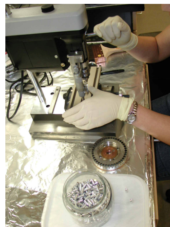
Fig. 6 Using lever to drill into UCI cathode.
