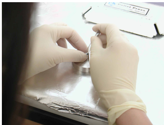
Fig. 7 Putting graphite into the cathode.
