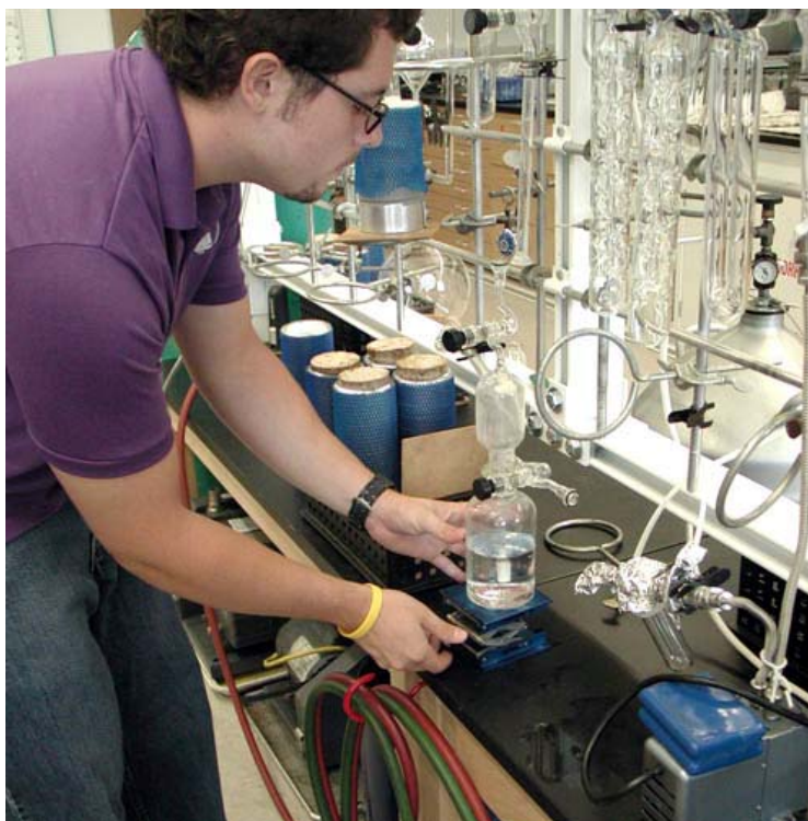
Figure 12. Bubbler being attached to line
