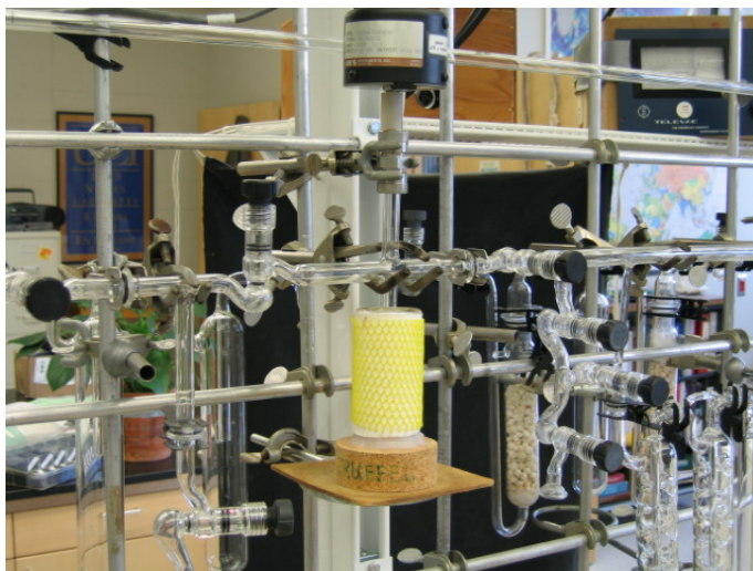
Figure 18. Small slush around measure volume
