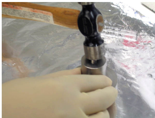
Fig.11 Using a hammer to pound the graphite.
