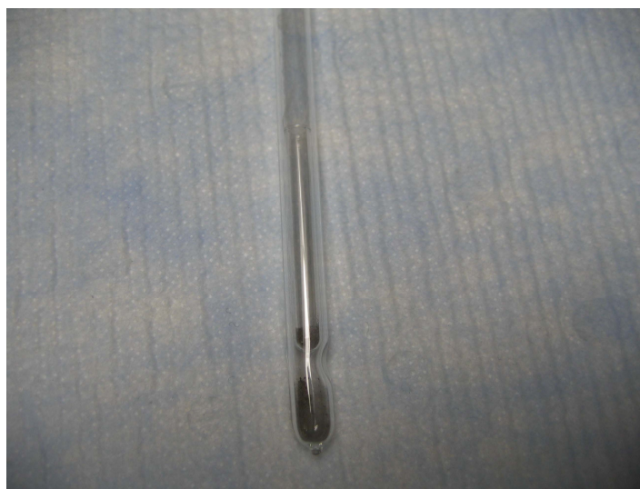
Fig. 6 Reactor of 9 mm Pyrex tube with 6 mm tube inside.
