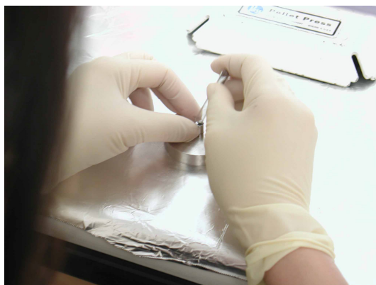
Fig.10 Putting graphite into the cathode.
