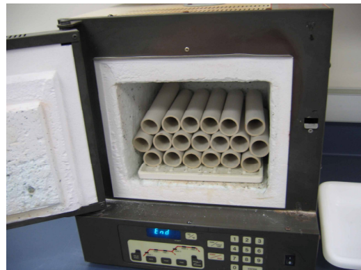
Fig. 5 NEY 2-525 furnace and ceramic tubes.
