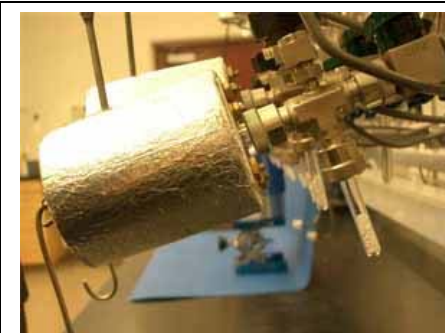
Fig. 4 Showing proper distance of the heater from the Ultra Torr fitting.
